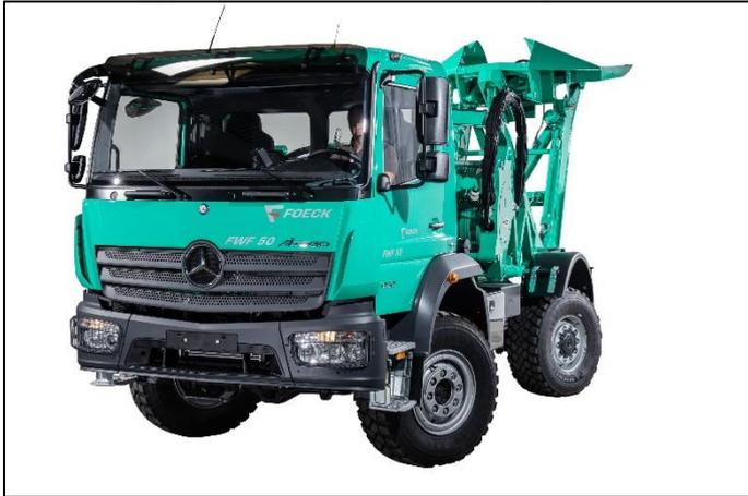
Bild 4. An ideal installation system: The new developed FWF 50 is perfectly suited as a pulling machine for the installation plough FSP 6.
