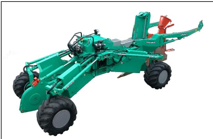
pic 3. The manoeuvrable laying plough FSP 6 can slim down to 1.95 m and, with a height of 2.91 m, can also pass through low passages.
