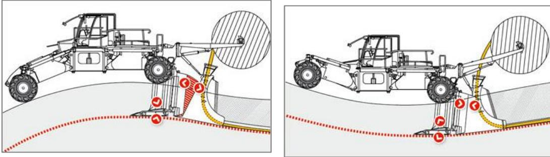
The ripper shoe, which can be adjusted by remote control, regulates the installation depth. This allows an exact laying on the prescribed bottom slope. Thanks to the multi-unit installation unit, tight curve radii of up to 3 m can be achieved.
