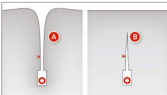
The laying material thus lies safely, without mechanical strain, after the laying process on the laying base smoothed by the FOECK Plough in the same work step.
