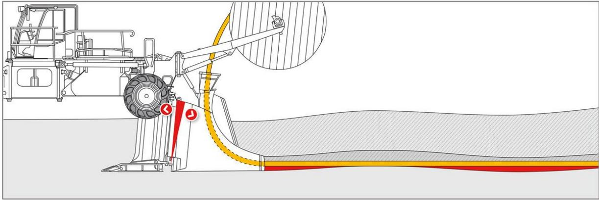
As this laying technology does not involve any ground subsidence caused by excavating and then subsequently compacting the earth, the cable or pipe is protected against mechanical strain for many years to come, as evidenced by long-term studies. Over time, fine particles which are washed in by the rain enclose the laid pipe or cable and provide additional protection.
