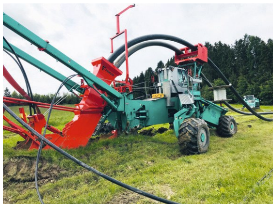
Laying extra-high voltage lines with the FSP 280, the most powerful laying plough with 360 t tractive force
