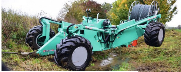
Powerful winch vehicle in action during the laying of fibre optic cables across a stream.
