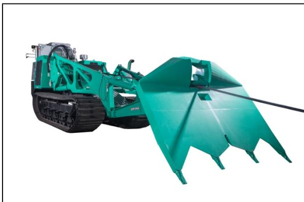
The FOECK Crawler with patented Schwenkmatic winch construction pulls the FOECK Plough with a constant force of up to 90 tonnes (in the pulley)
