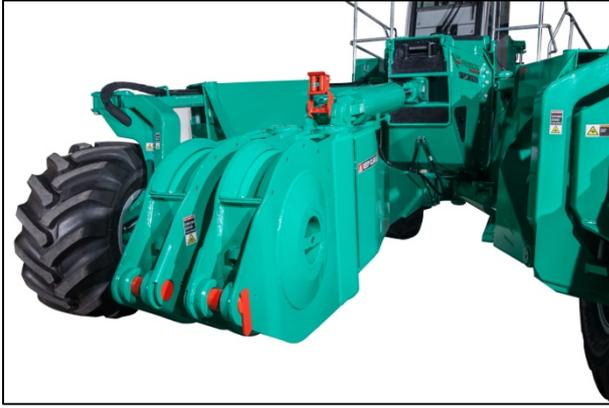
With the double drawbar, the FSP 280 laying plough can be pulled in parallel by two winch vehicles with up to 360 tonnes (2x pulley)
