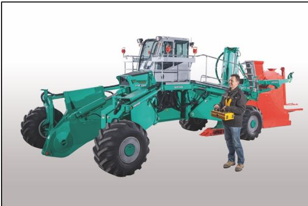
**With the new remote control system, the FOECK laying plough can now also be fully operated from outside the vehicle**
